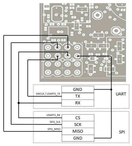
Note: As you see, the UART RX and SPI CS use the same shared pin. The function of this pin (UART receiver, SPI chip select or others) can be selected in dashboard by parameter 'PA15 pin function' in 'Interfaces' section.
