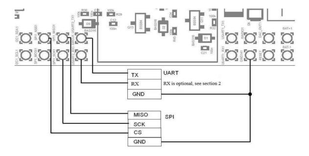
The hedgehog constantly streams packets of location data, defined in section 1, to UART and USB without any request. To get data from SPI, master should provide signals of chip select (CS) and clock (SCK).
